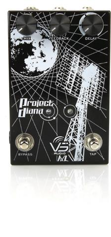
analog audio path delay, featuring tap tempo, five different subdivisions and 600ms maximum delay time. Designed with custom analog anti-aliasing and reconstruction filters, the four original Panasonic MN3008 BBD chips produce warm tight slap back echoes and long deep end delay tones.
